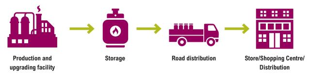
When transported by trucks, biomethane is usually carried or stored in high-pressure cylinders in a range from 200 bar to 250 bar. This option is more energy and cost intensive due to additional operations added to the value chain. This process is more commonly used for long distance transport, such as by heavy duty vehicles or maritime transport.<sup>52</sup>
